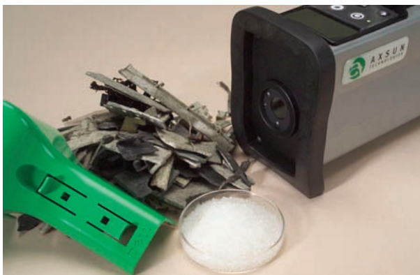
Figure 3. To identify materials, the Anavo is pressed up against the sample, and an answer is given in less than one second.
